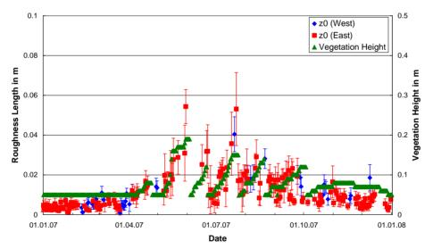
Figure 4 Time evolution of the estimated values of mean vegetation height (right yaxis) and roughness length for momentum (left y-axis) at the Falkenberg boundary layer field site for the 2007 annual cycle (red and blue symbols indicate estimates based on measurements at the two flux stations in the eastern and western part of the field site – see section 2)
